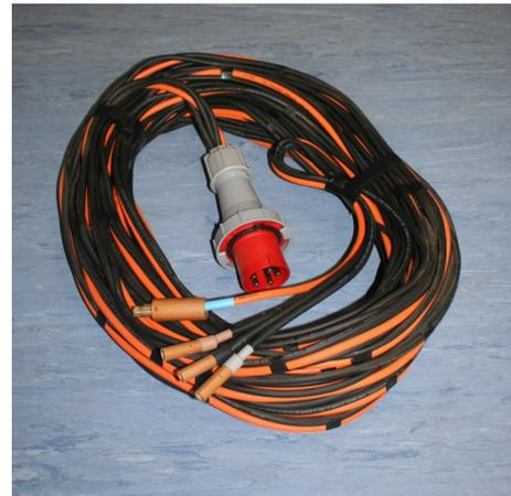
The quad cable set consists of four lengths of heat and oil resistant flame retardant (HOFR), double insulated copper cable, three of the lengths are made of black copper cable and one length from orange copper cable. There are three 60 amp female twistlocks and one 300 amp male twistlock at one end and a five pin 415 volt plug attached at the other end for connection to the mains or distribution unit.
